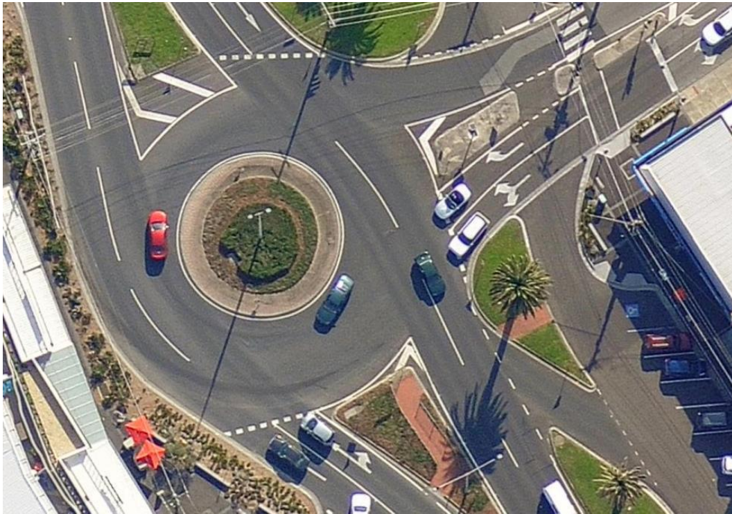
Figure 7-3: Roundabout Metering Using Pedestrian Operated Signals on Approach Leg only and Zebra Crossing on Exiting Leg
