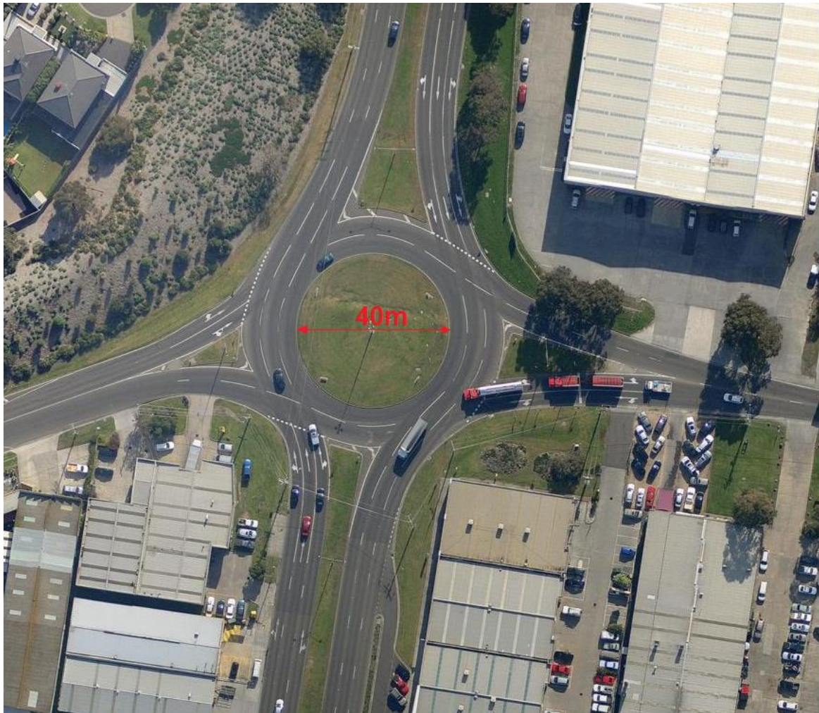
Figure B.2: Example of 3-lane Roundabout in Victoria (Boundary Rd / Governor Rd, Braeside)
